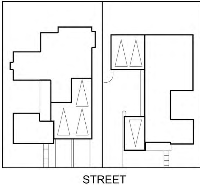
CONCEPTUAL BUILDING TYPE A & LOT SIZE: Single-Family Detached Front Loaded (60'x100') (subject to future City approvals)
